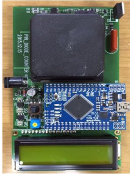
Figure 2. Implemented PIN photodiode radon counter
